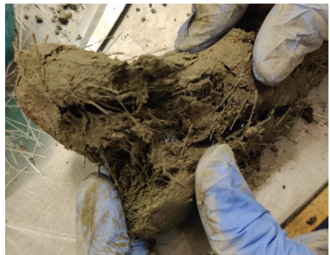
Figure 5: Fresh concrete showing air bubbles that are created due to foaming agent
