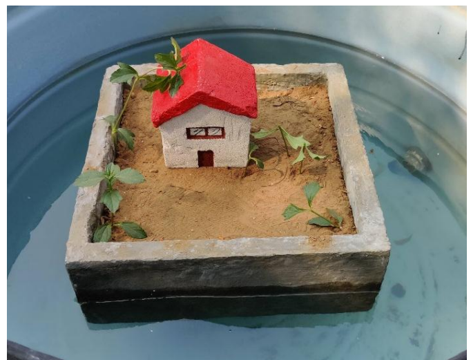
Figure 9: Scaled model for floating platforms with house.
