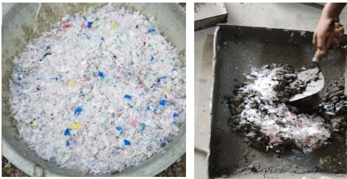
Fig. 1: Mixing of shredded waste plastic with concrete
