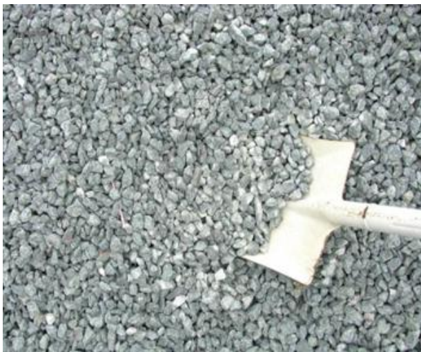
Fig - 2: Crushed coarse aggregate (20 mm)
