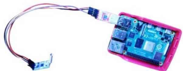
Fig.2 LoRa HC-12 interfaced to Raspberry Pi 4 using CP2102
