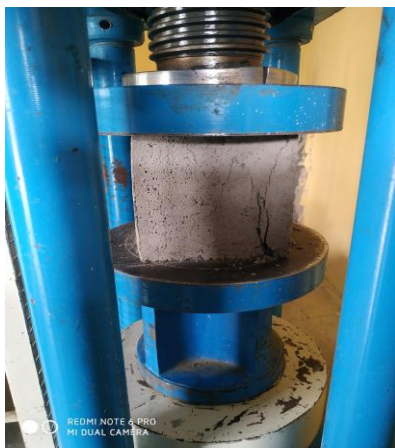
Fig -7: Concrete Testing on Compression Testing Machine
