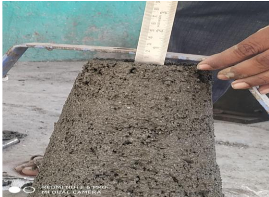
Fig-6: Slump Cone Test
