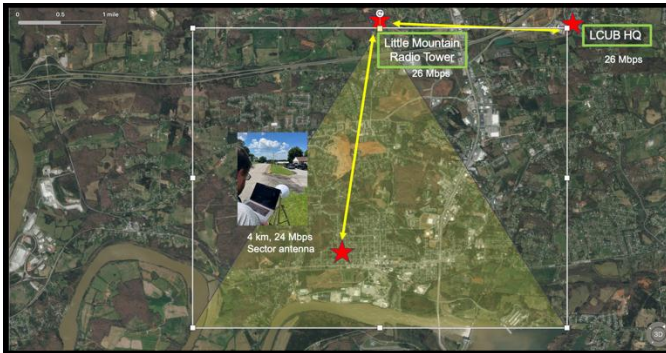
Fig. 13. In-field data throughput measurements for the PtMP configuration.
