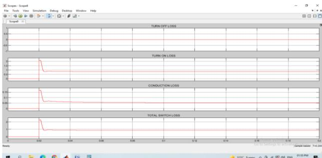
**Fig 18:** Switching losses of Interleaved boost converter
