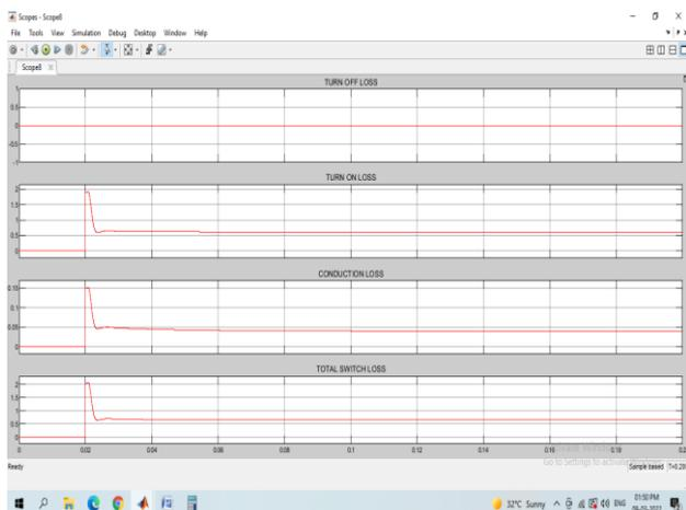
**Fig 12:** Switching losses of Interleaved boost converter
