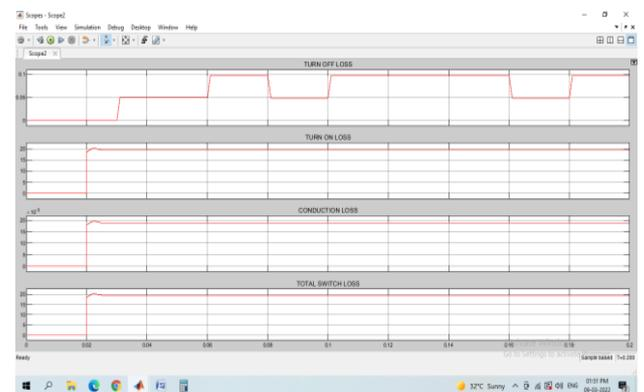
**Fig 14:** The inverter switch losses
