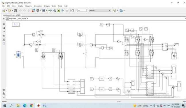
**Fig 16:** Simulation circuit of conventional three phase system
