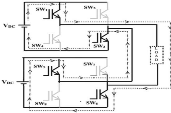
Fig 5: Mode 1 equivalent circuit of 5 level CHBMLI
