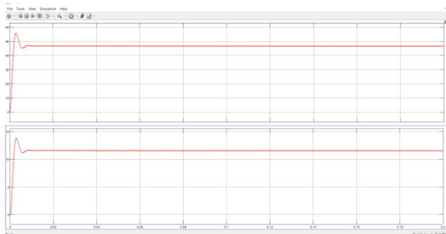
**Fig 17:** Interleaved boost converter output voltage and current
