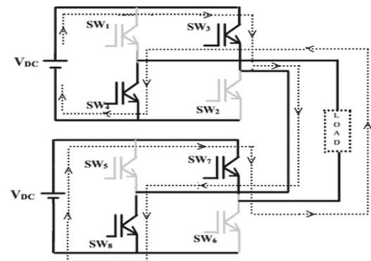
Fig 9: Mode 5 equivalent circuit of 5 level CHBMLI
