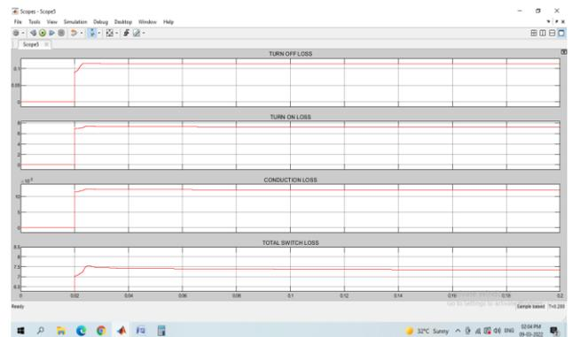
**Fig 26 :** Switching losses of 5 level inverter
