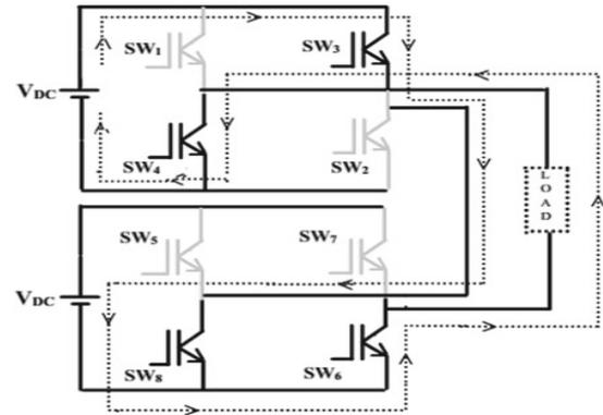
Fig 8: Mode 4 equivalent circuit of 5 level CHBMLI
