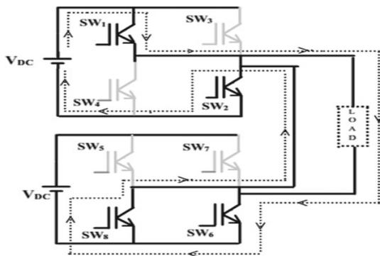
Fig 6: Mode 2 equivalent circuit of 5 level CHBMLI
