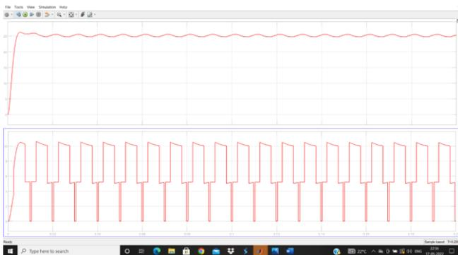
**Fig 23:** Interleaved boost converter voltage and current
