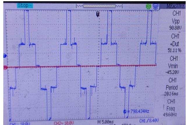
Fig 29 : 5 level Inverter voltage
