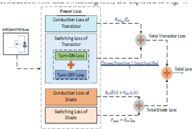
**Fig 2:** Power loss model of inverter
