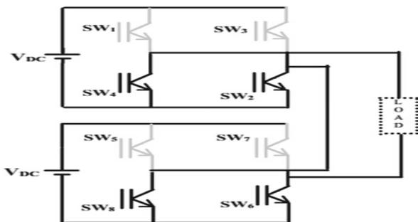
Fig 7: Mode 3 equivalent circuit of 5 level CHBMLI
