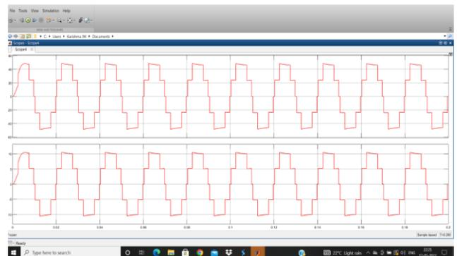
**Fig 25:** Inverter load voltage and current
