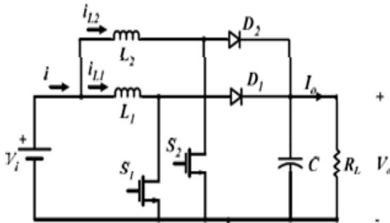
**Fig 3:** Circuit configuration of interleaved boost converter
